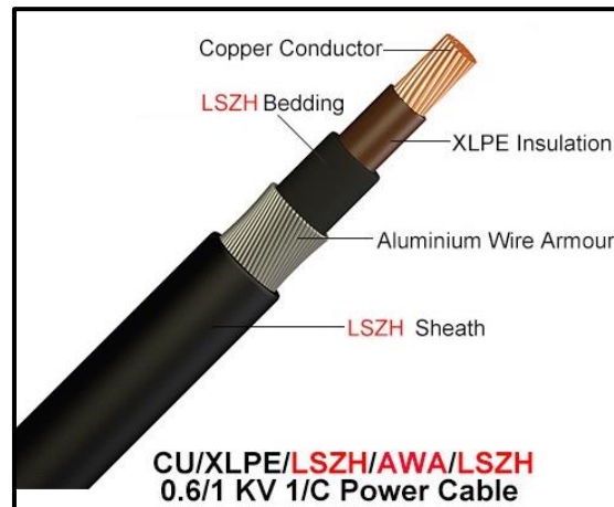
Fig.1.11 constructional parts of LSZH Fire rated cable
