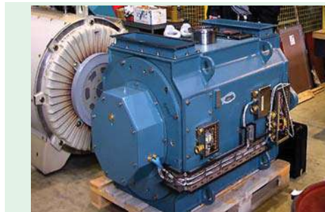
Induction motor for drilling applications
